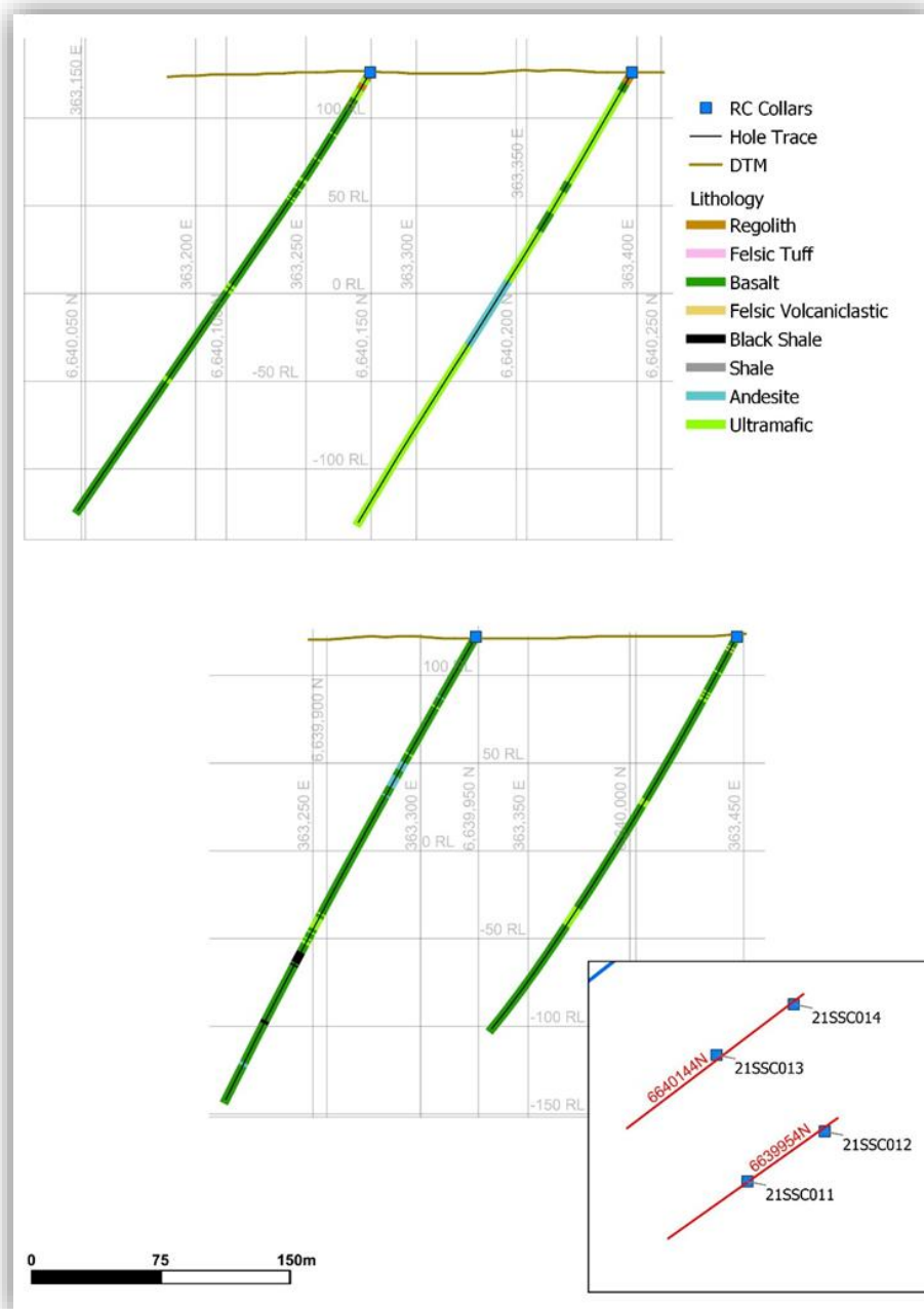
Figure 5: Cross section (Looking NW) of RC drilling at Wise Ni target
