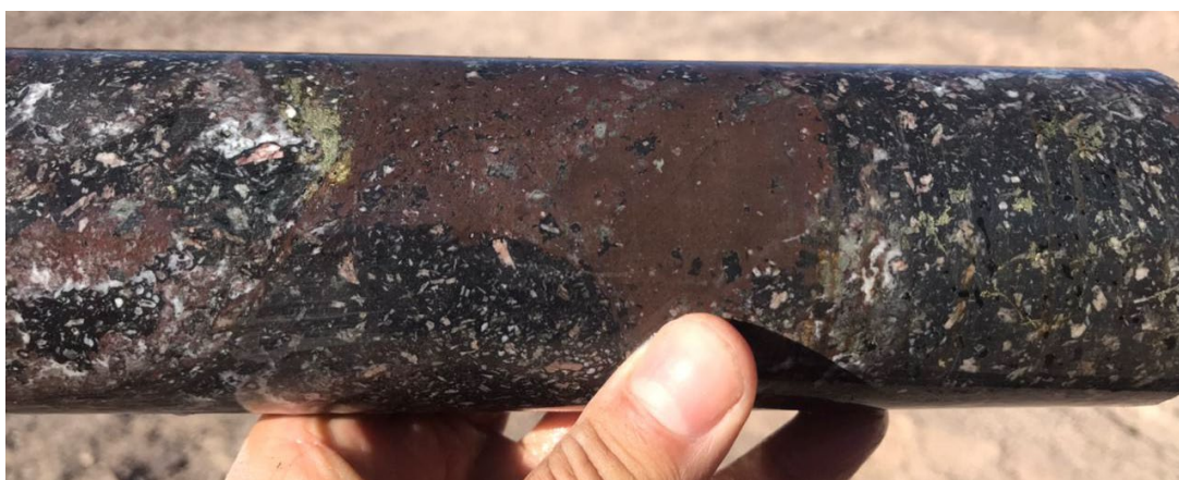
Figure 3: Mostazal Copper Project – diamond drill core from MODD001, showing altered porphyritic andesite host rock with disseminated and clotty sulphide mineralisation, including pyrite and chalcopyrite (copper sulphide)
