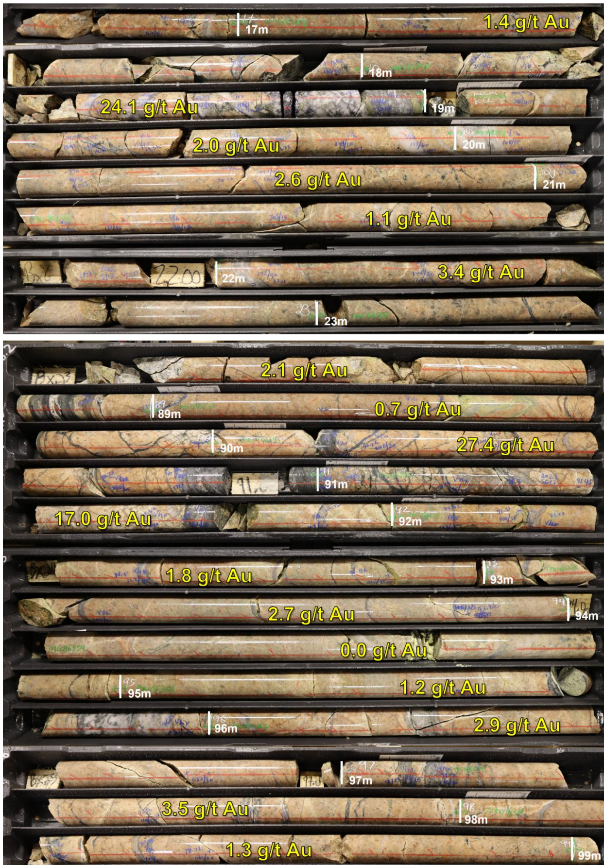
Figure 6: High grade gold association with increased density and width of sulphide-rich quartz stockwork and sheeted veins in CRD318
