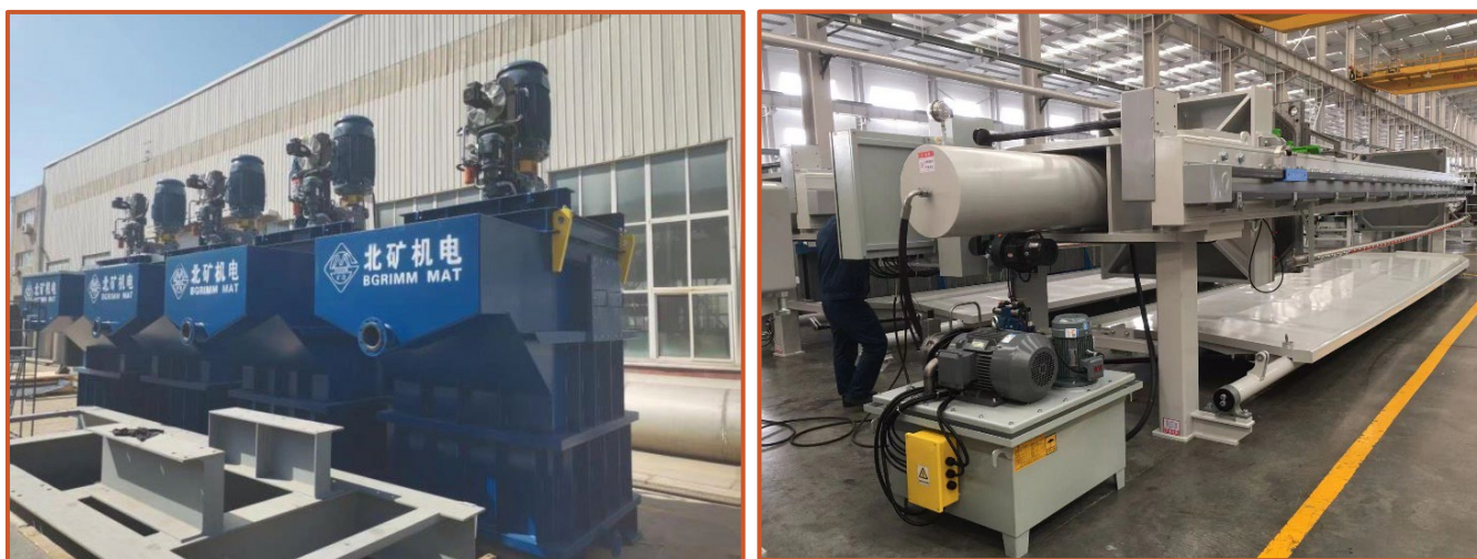
Figure 2: Factory acceptance tests of the BGRIMM attritioning mills (left) and filter press (right).
