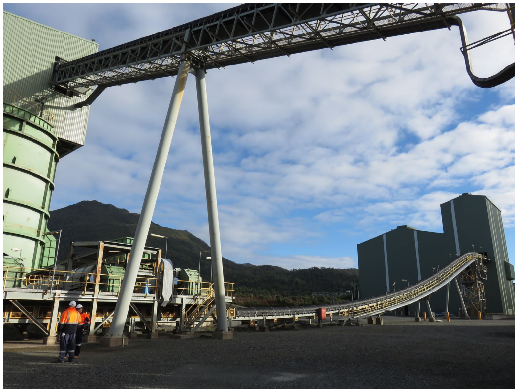
Figure 7. Conveyors to crusher (upper) and from fine ore bin to concentrator (lower)
