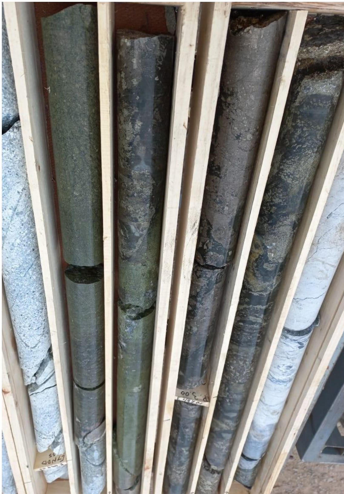
Photo 3 - GNDD-555 : Massive sulphides and skarn alteration logged (495.1-498.7m)
