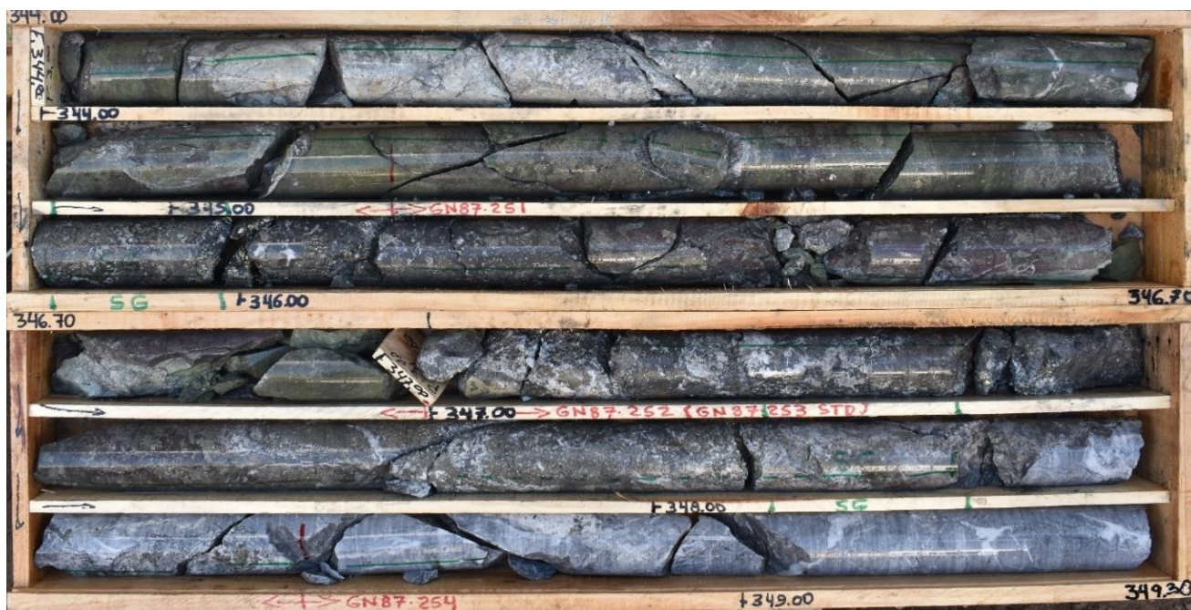
Photo 6 - GNDD-545 : Massive sulphides and skarn alteration logged (343.0-348.3m)
