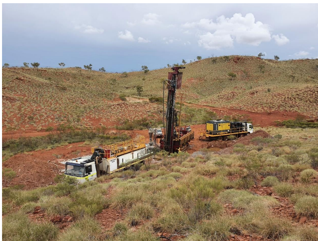
Photograph: Reverse Circulation (RC) drill rig at the Ayshia Prospect
