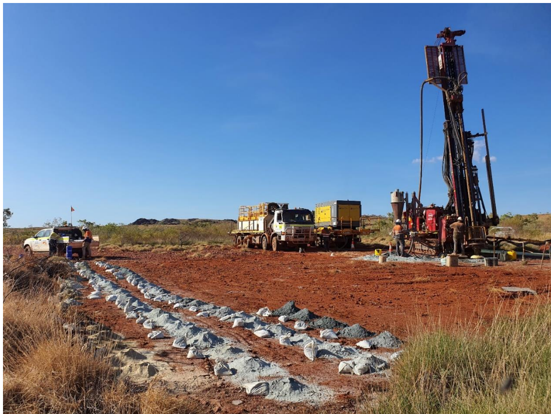
Photograph: Reverse Circulation (RC) drill rig at the Whundo Copper mine
