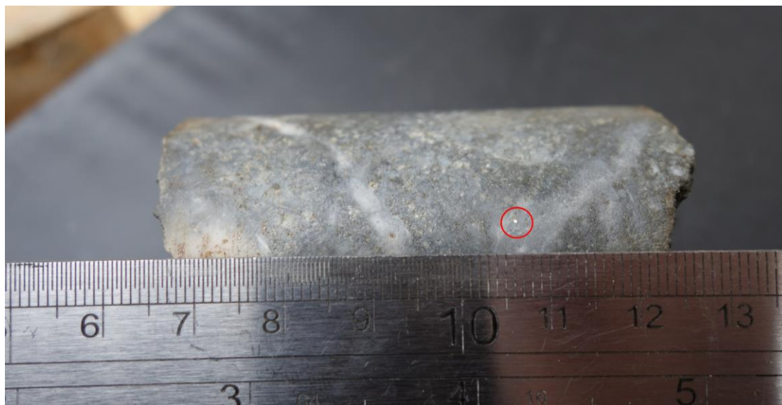
Figure 6: Drill core photo of the visible gold at 68.7m in UGA-30, in a 5-7mm wide, white to grey chalcedonic quartz-pyrite filled vein within a stockwork zone.
