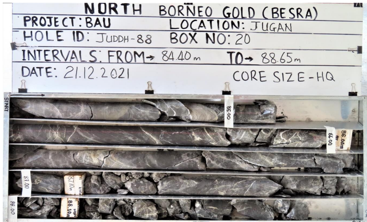
Figure 7: Core recovered from JUDDH-88 for portion of the interval 82m-88m @5.98 g/t Au, proximal to the interpreted footwall thrust.
