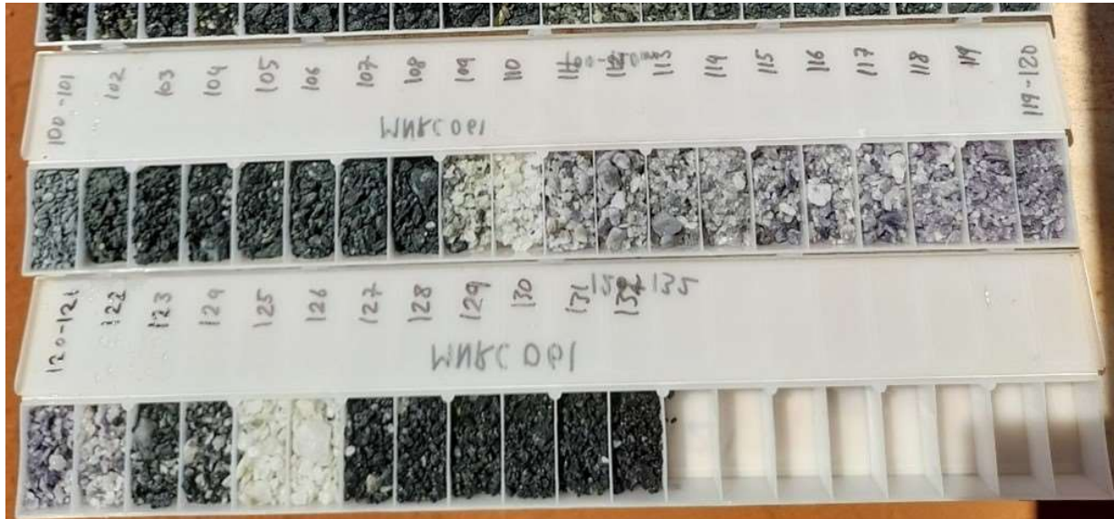
Photo 1: Intersection of LCT pegmatite from 109m to 126m in MNRC061 with purple Li-Rb bearing minerals
