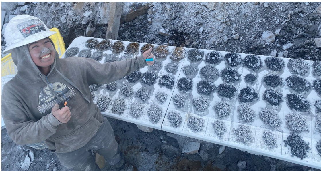
Figure 1. RC drill chips laid out for logging at Star Canyon, Humboldt Range, Nevada. Note intense bleaching of the lower two rows of samples.
