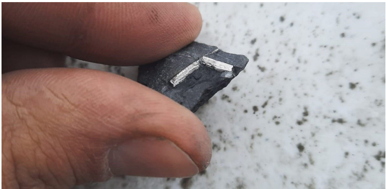
Figure 6. Stibnite (antimony sulphide) crystals in silicified silty limestone in RC drill chip, Star Canyon.
