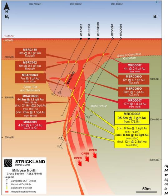
Figure 1: Millrose cross section showing high grade depth extension in hole MRDD008.
