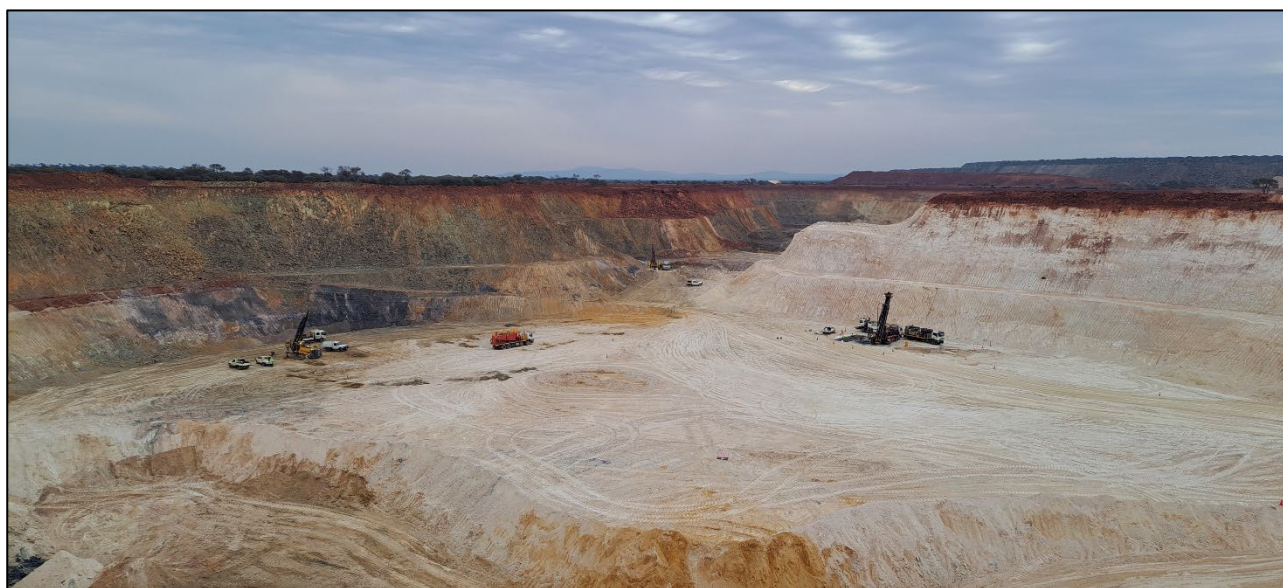
Figure 4: Three drill rigs in the Plymouth open pit looking southwest. The small RC rig on the left is drilling the Plymouth East-West lodes running parallel to the colour change with the Sly Fox pit outside frame to the left, the diamond drill rig is in the centre background testing the intersection between the Plymouth East-West and North-South lodes and the large RC rig on the right is drilling the Plymouth North-South lodes as they head up the eastern side of the Gilbey's open pit.
