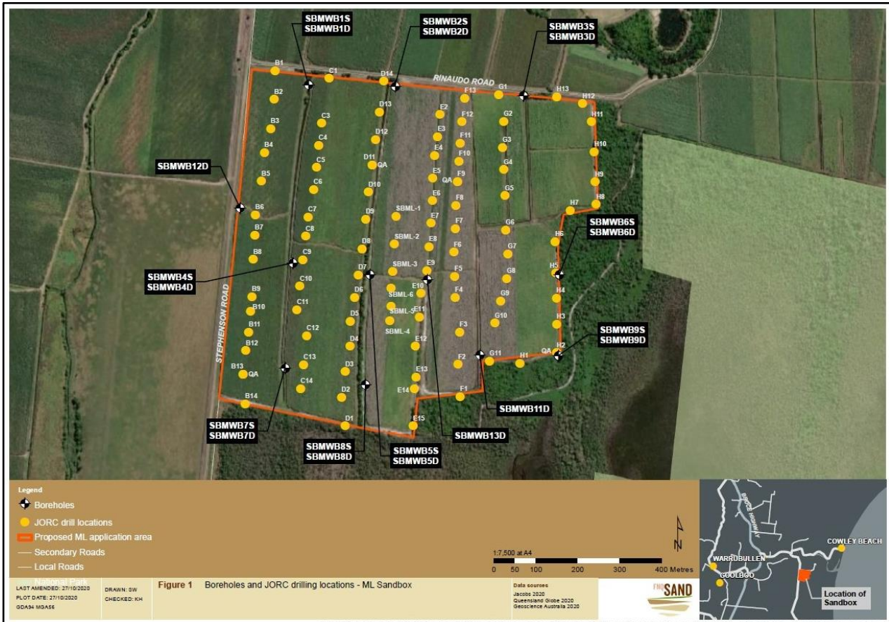
Figure 4: Drill Collar Plan for Sandbox (IPA)
