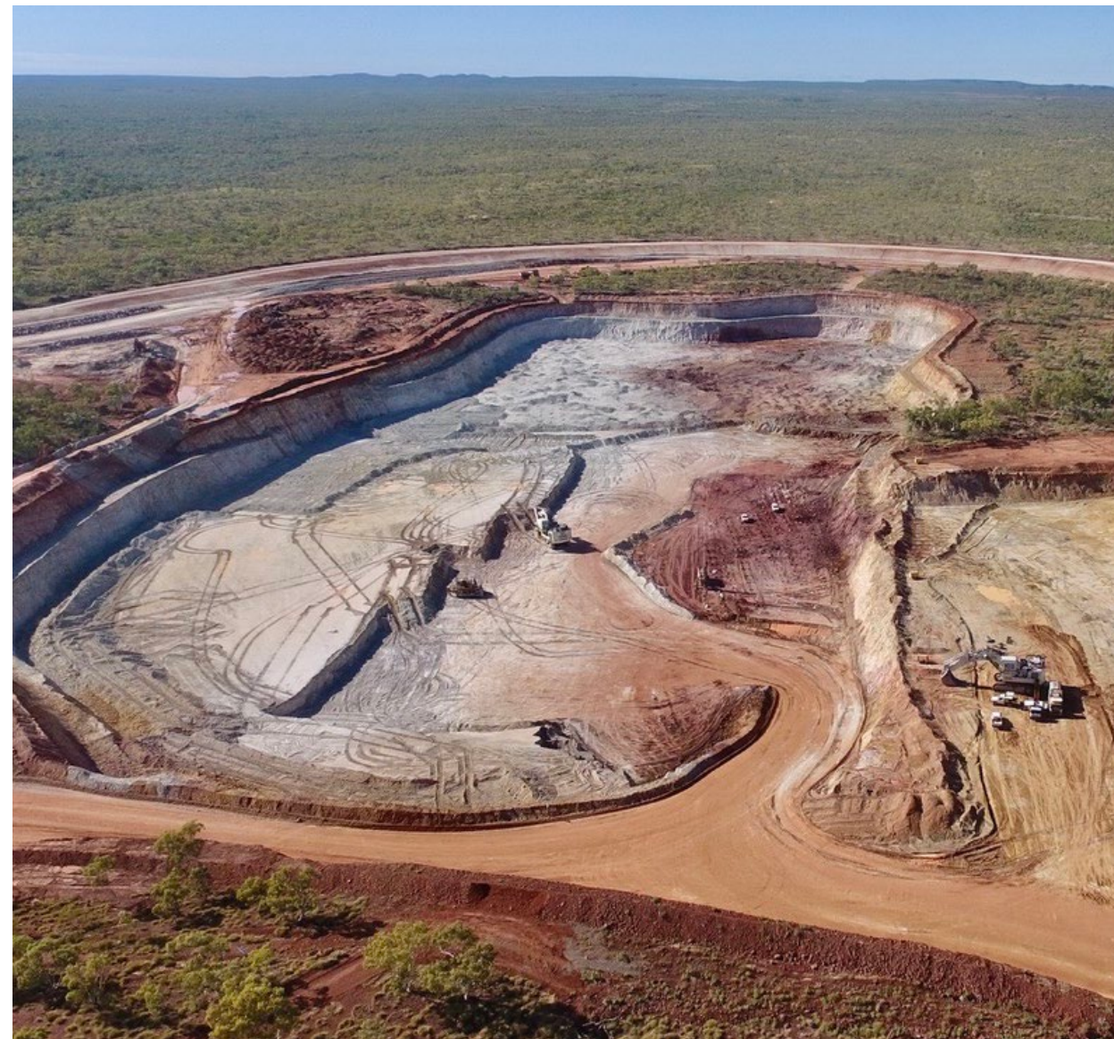
Mining at east pit 27 Apr 22. Ore can be seen on RHS of pit as darker coloured material.
