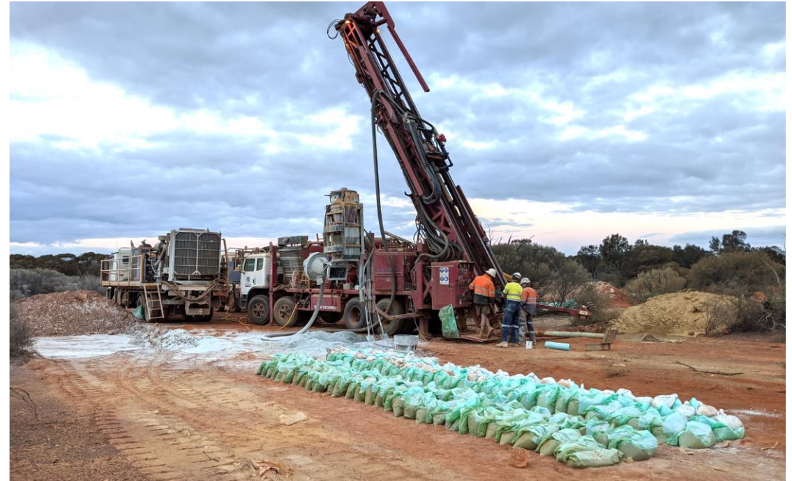
Figure 10: RC drill rig onsite at Mulgabbie
