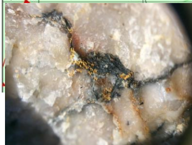
NQ drill core, 47.6mm diameter
