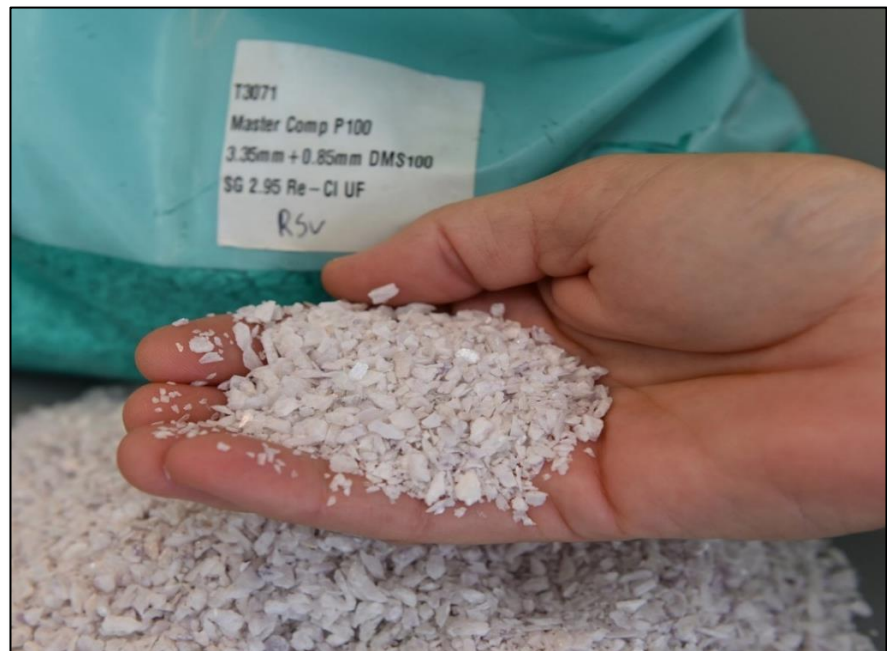
Figure 1; Spodumene DMS concentrate produced from 3.35mm-+0.85mm DMS 2.95 feed
