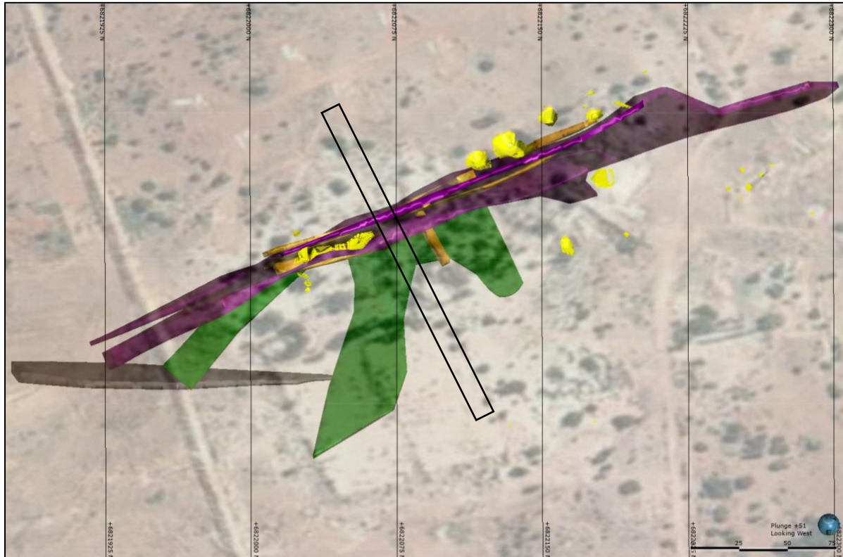
Figure 6: View west and down plunge of Euro North Main Zone high-grade structures (magenta). The flat-dipping footwall structure is coloured green and moderate west-dipping structure coloured grey. Surface expression of shafts are yellow polygons. Modelled mining voids are orange coloured. Section box for Figure 7 is marked.
