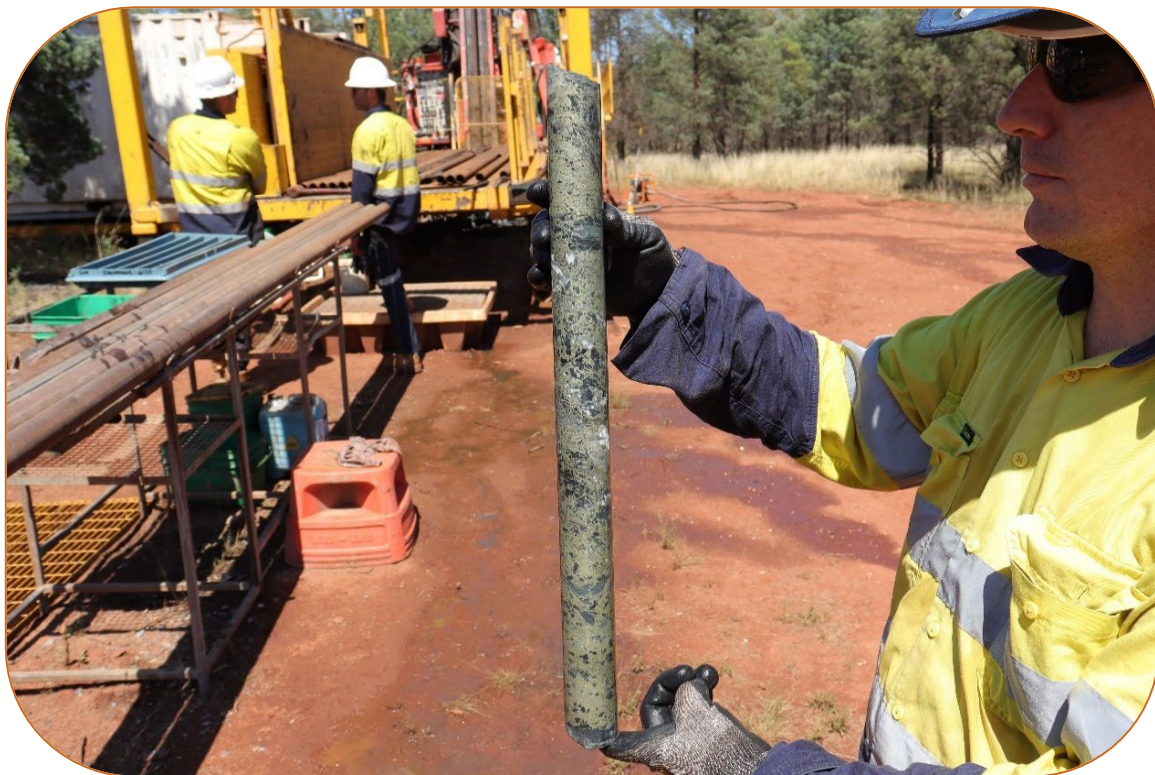
Figure 1 – Massive to semi-massive chalcopyrite intersected from 425.2 metres in CANDD006
