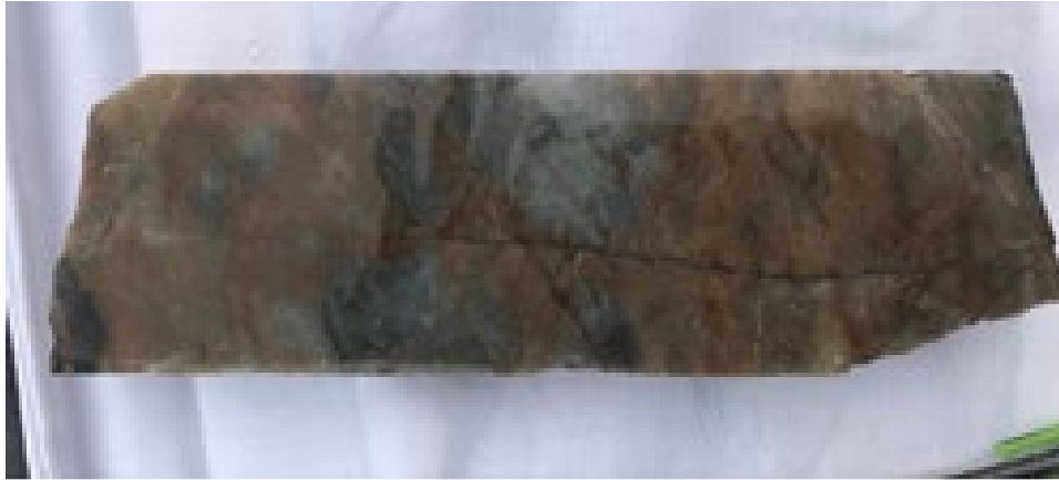
Photo 1 - WD002, 185.9m Altered pale brown silica/ jasperoid replaced sediment. Anomalous in Ag +/- Sb, Tl & W
