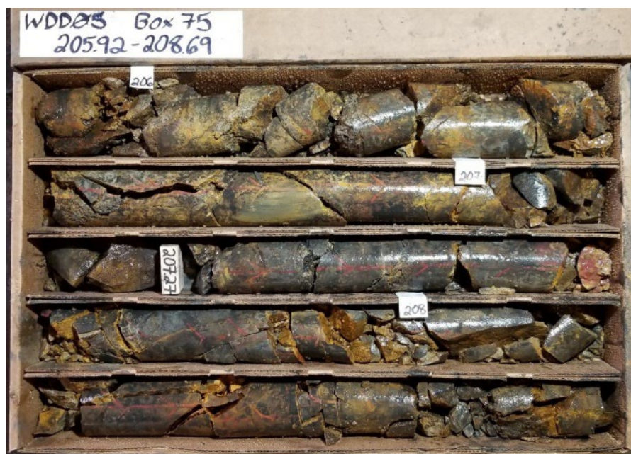
Figure 4 - WD005 – Altered, oxidised and brecciated shale. Anomalous in Ag, As, Sb, Te +/- Hg
