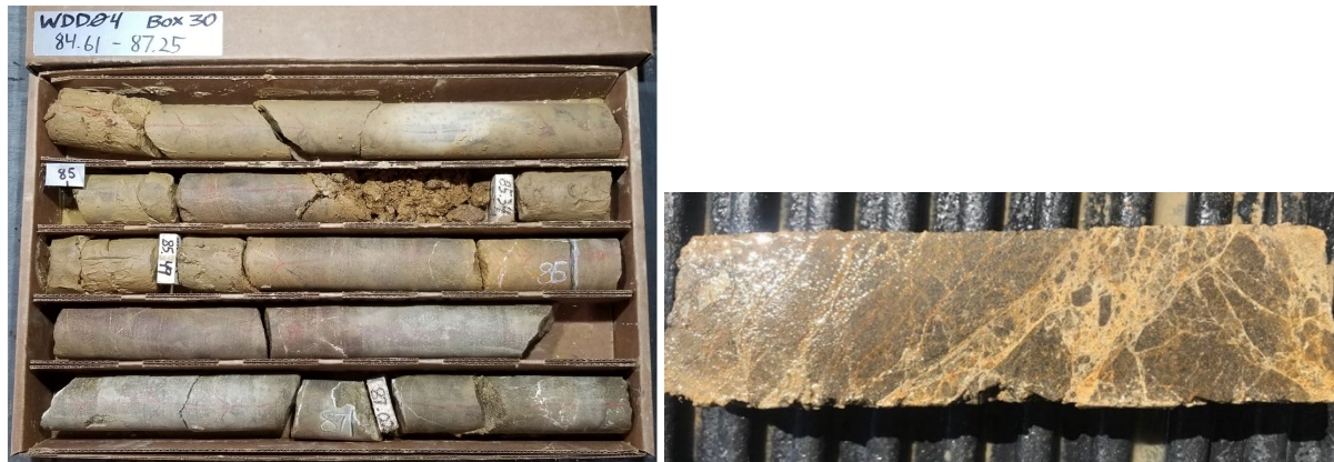
Figure 5 – Altered, oxidised and brecciated lamprophyre dyke (WD004)
