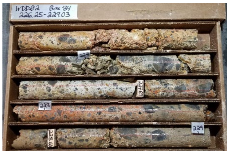
Photo 3 - WD002, oxidised conglomerate/fault breccia (WD002), anomalous in Ag, +/- As, Ba and Sb
