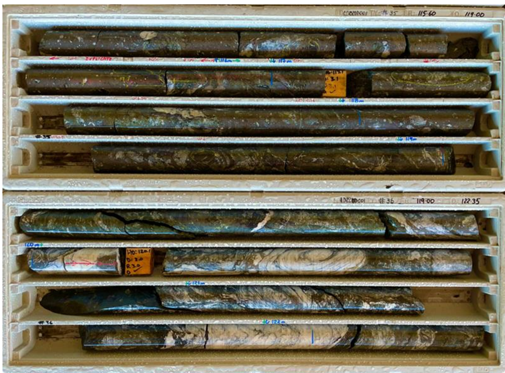
Figure 5: LD22DD001 from 115.6 – 122.35m – intervals of massive sulphide with chalcopyrite + pyrrhotite and quartz – carbonate hydrothermal breccia and veining.
