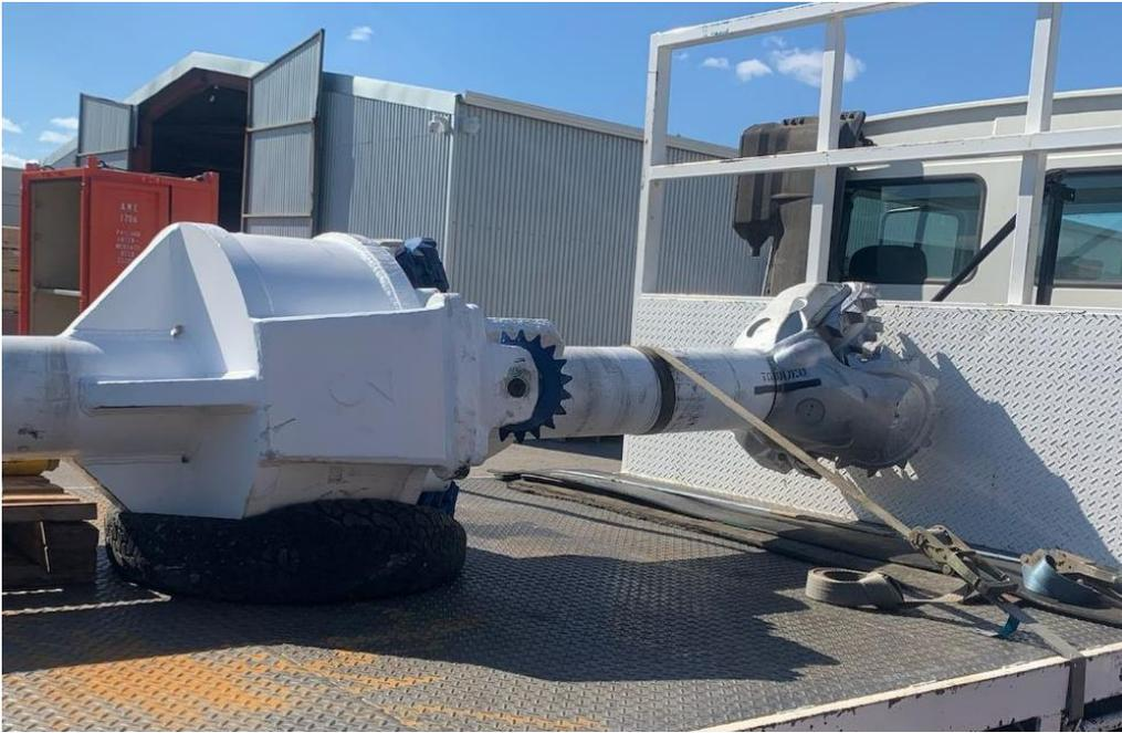
Hole Opener 26" Bit x 42" Hole Opener
