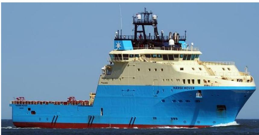
Maersk Mover Anchor Handling Supply Vessel (AHSV)
