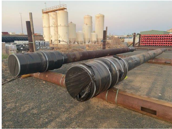
High Pressure Wellhead Housings (HPWHH)
