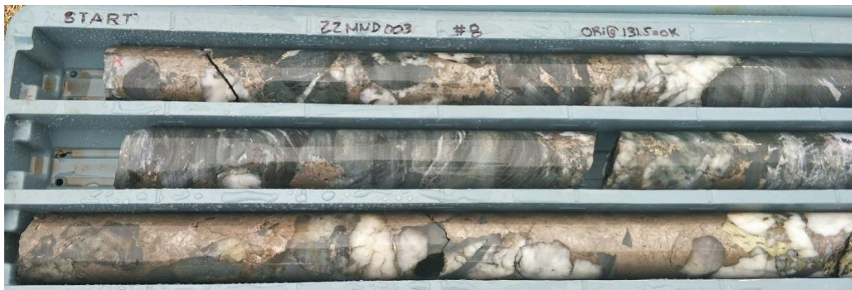
Photo 1: 22MNDD003 tray #8 with massive pyrrhotite and chalcopyrite quartz-carbonate breccia veins hosted in dolerite with 1m @ 21.30g/t (130m) shown at the bottom of the photo
