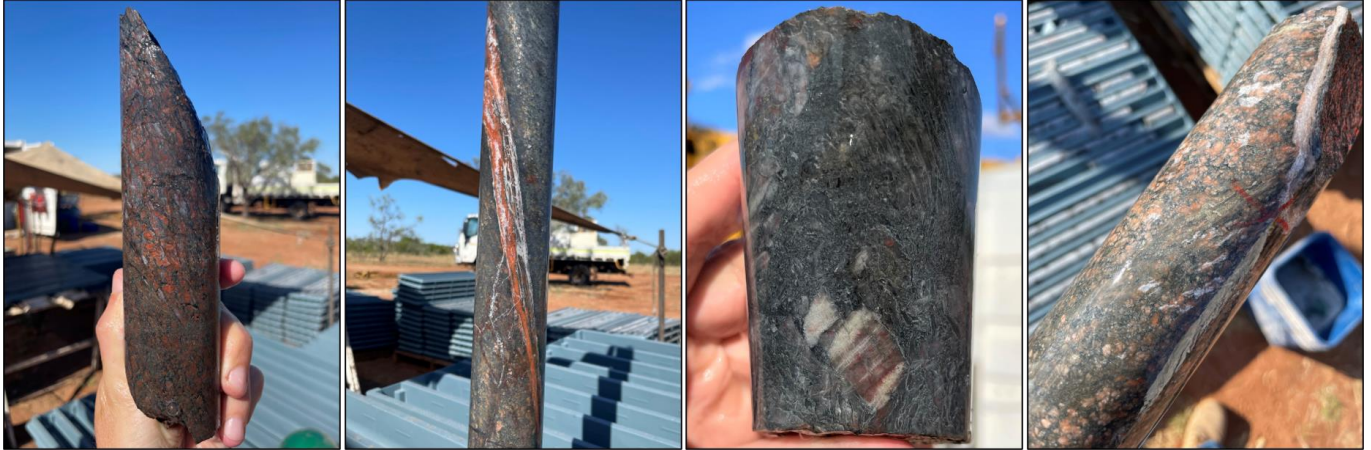
Figure 4: Core photos taken rig-side at FW220001 from 833 to 840m down hole depth. Left: Strongly haematite altered granite with abundant fracturing and quartz veinlets. Centre Left: Chlorite-epidote-haematite altered granite with multiple phases of veins and fracturing overprinted by a younger potassium feldspar rich vein. Centre Right: Quartz-haematite altered clasts in a silicified fault/breccia zone. Right: Minor levels of pyrite disseminated throughout a potassium feldspar-haematite altered zone with quartz-carbonate-(potassium feldspar) veins.
