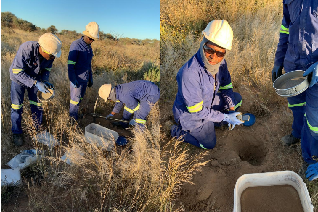
Figure 4: Ground team collecting and plotting samples on 100m lines for in-fill soil survey at Daheim ahead of next round of drilling
