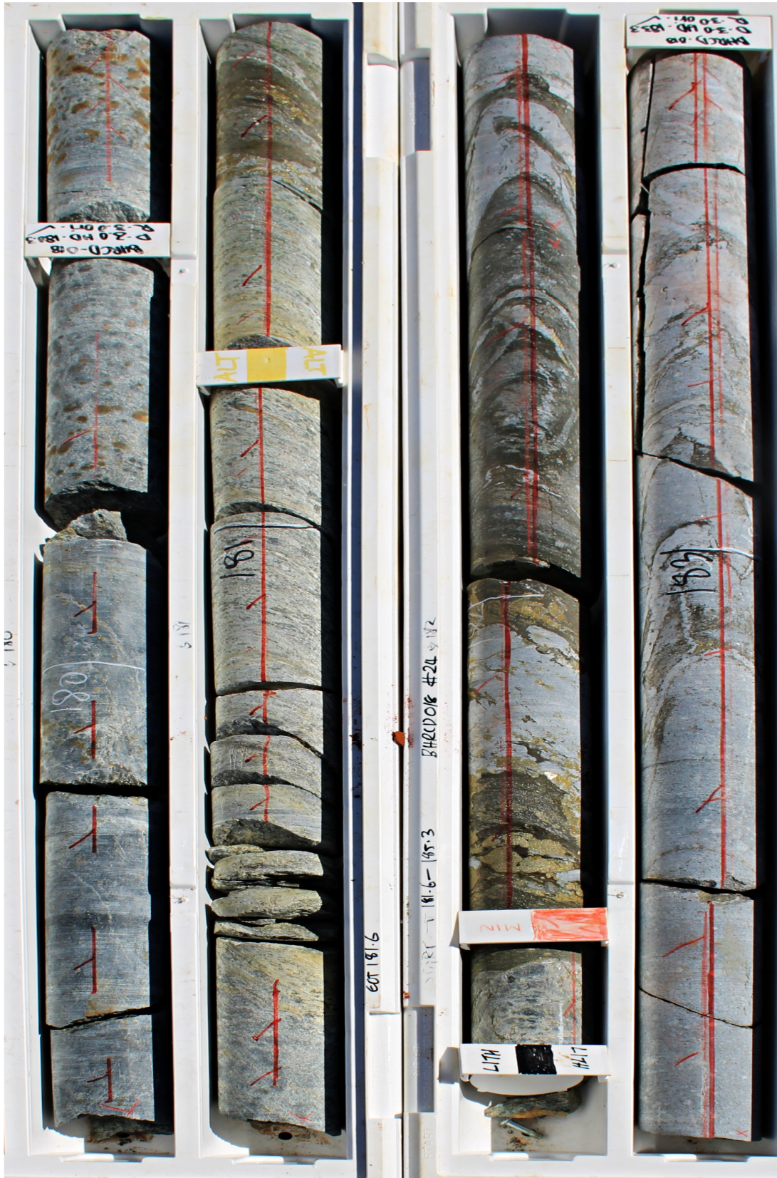
Figure 4: BHRCD018 core from 179.7m – 181.7m, showing massive and blebby sulphides through altered ultramafic
