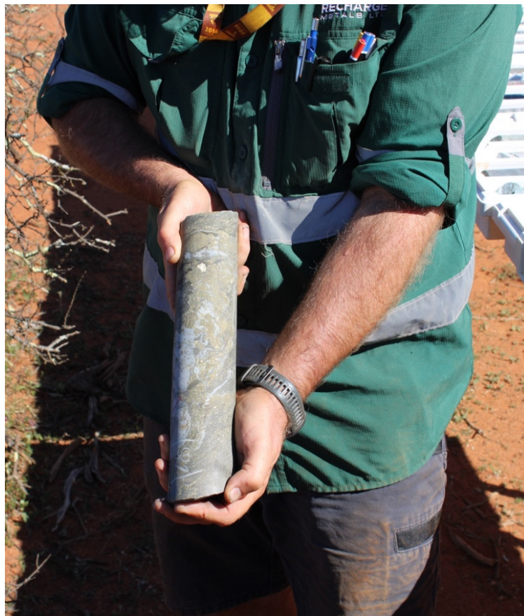
Figure 3: BHRCD018 core from 181.4m, showing massive and blebby sulphides through altered ultramafics
