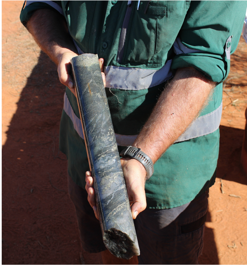
Figure 5: BHRC018 core from 335.4m, showing blebby sulphides through altered Andesite/Gabbro
