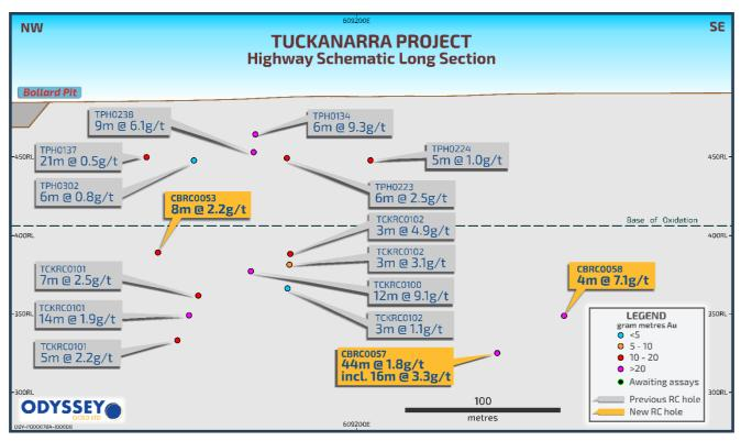
Figure 1. Highway Zone Long Section. Results from this announcement in yellow.
