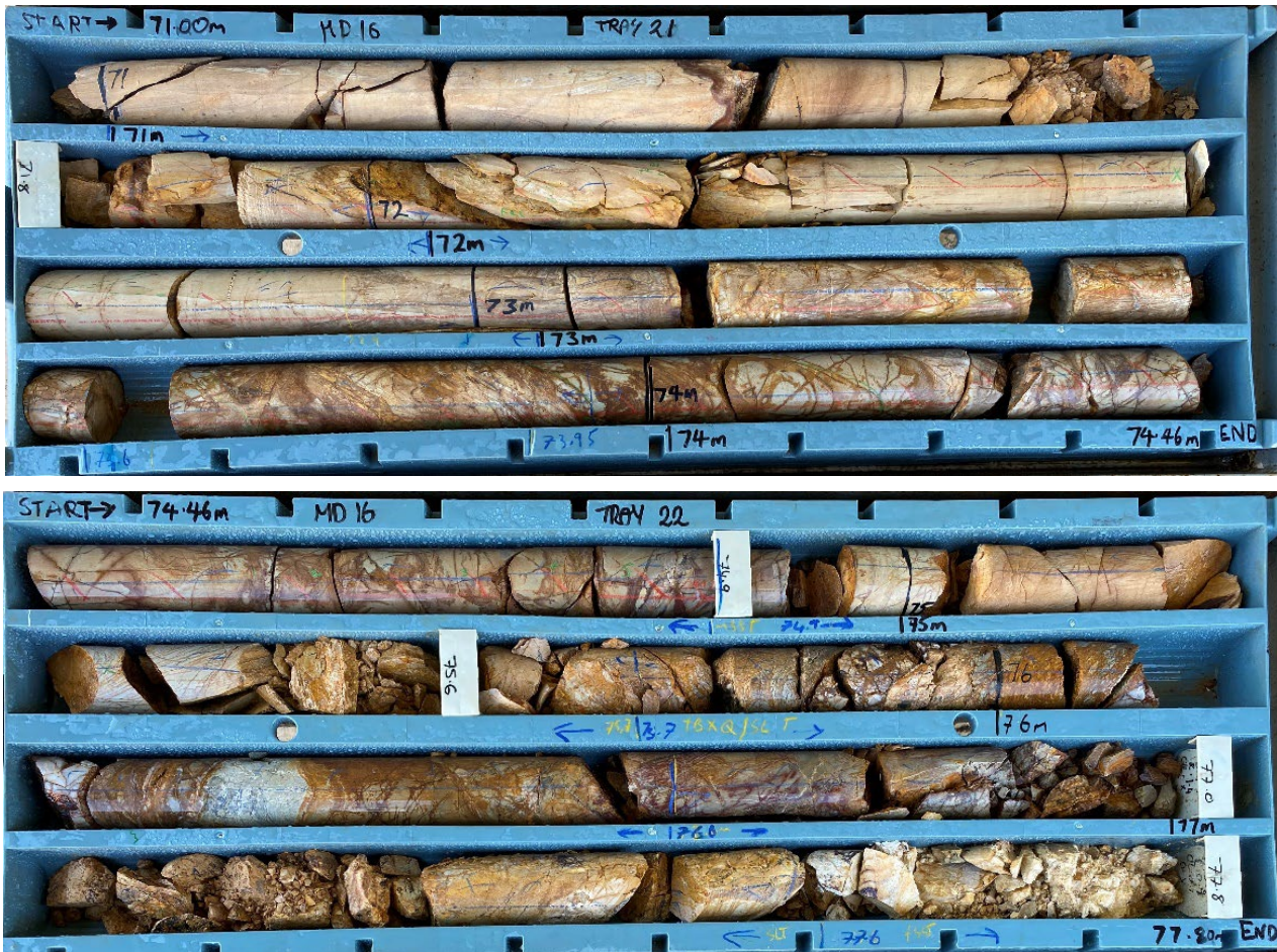
Figure 5: MD16 Tray 21, 22 & 23. Oxidised upper Leven Star intersection. 6.8 m @ 2.5 g/t Au from 73 m incl. 1.3 m @ 5.6 g/t Au from 73.6 m & 0.9 m @ 8.7 g/t Au from 75.7 m. Limonitic tectonic fault breccia (TBXH). Interval ends in 1.1 m of core loss.
