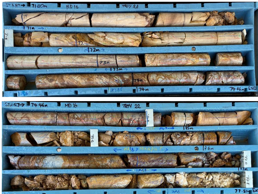
(Figure 4: MD16 Tray 21, 22 & 23. Oxidised upper Leven Star intersection. 6.8 m @ 2.5 g/t Au from 73 m incl. 1.3 m @ 5.6 g/t Au from 73.6 m & 0.9 m @ 8.7 g/t Au from 75.7 m. Limonitic tectonic fault breccia (TBXH). Interval ends in 1.1 m of core loss.)
