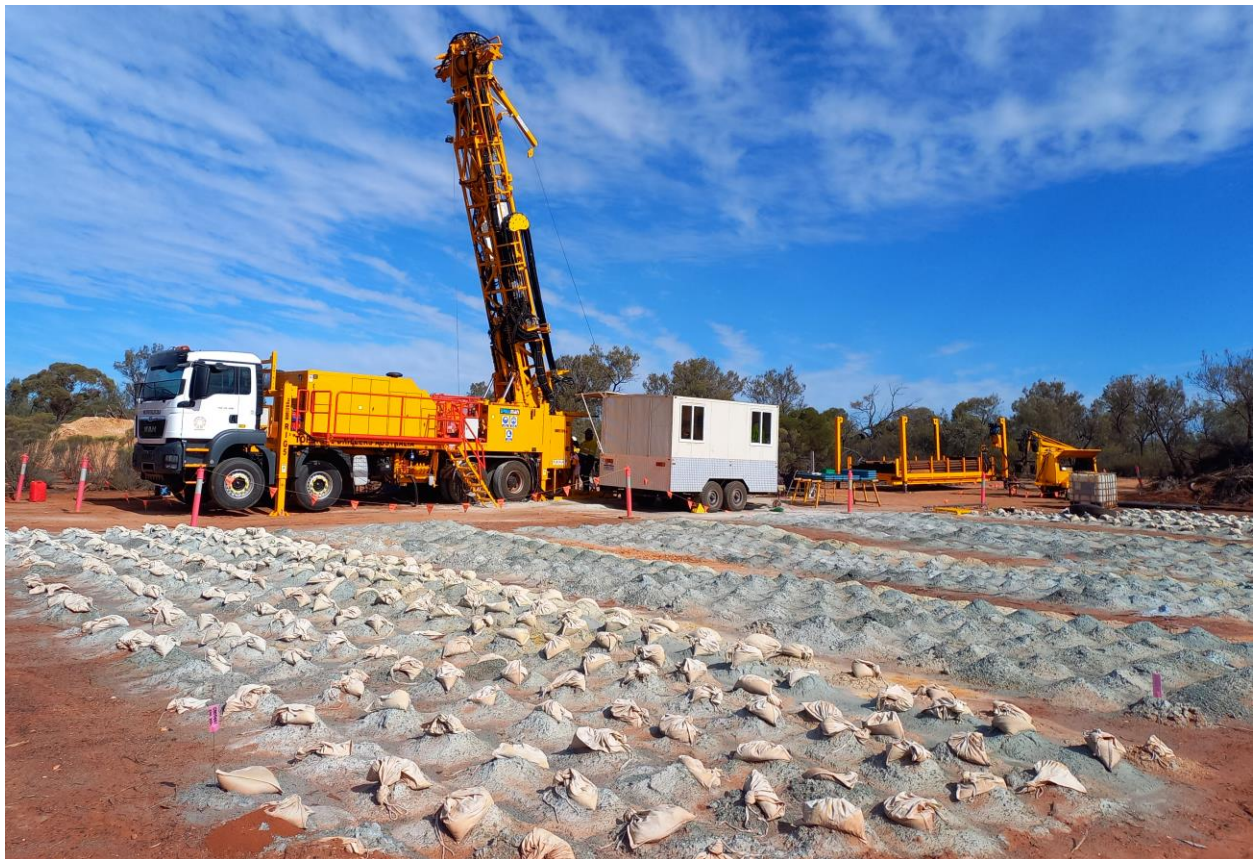
Figure 1. New UDR1200 diamond drill rig being commissioned at the T5 Ni-Cu Sulphide Prospect.
