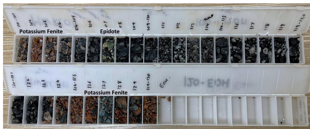
Figure 1: Sample trays from drill hole MWRC011 at MW2 showing potassic fenitisation and epidote alteration. The area of alteration hosts magnetite, calcite and apatite veins.
