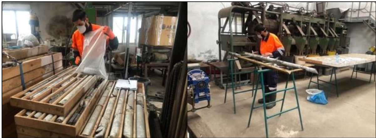
Figure 3. Drill core samples in plastic bags for shipment. Orienting drill core for structural purposes at Finx Sn-W mine.
