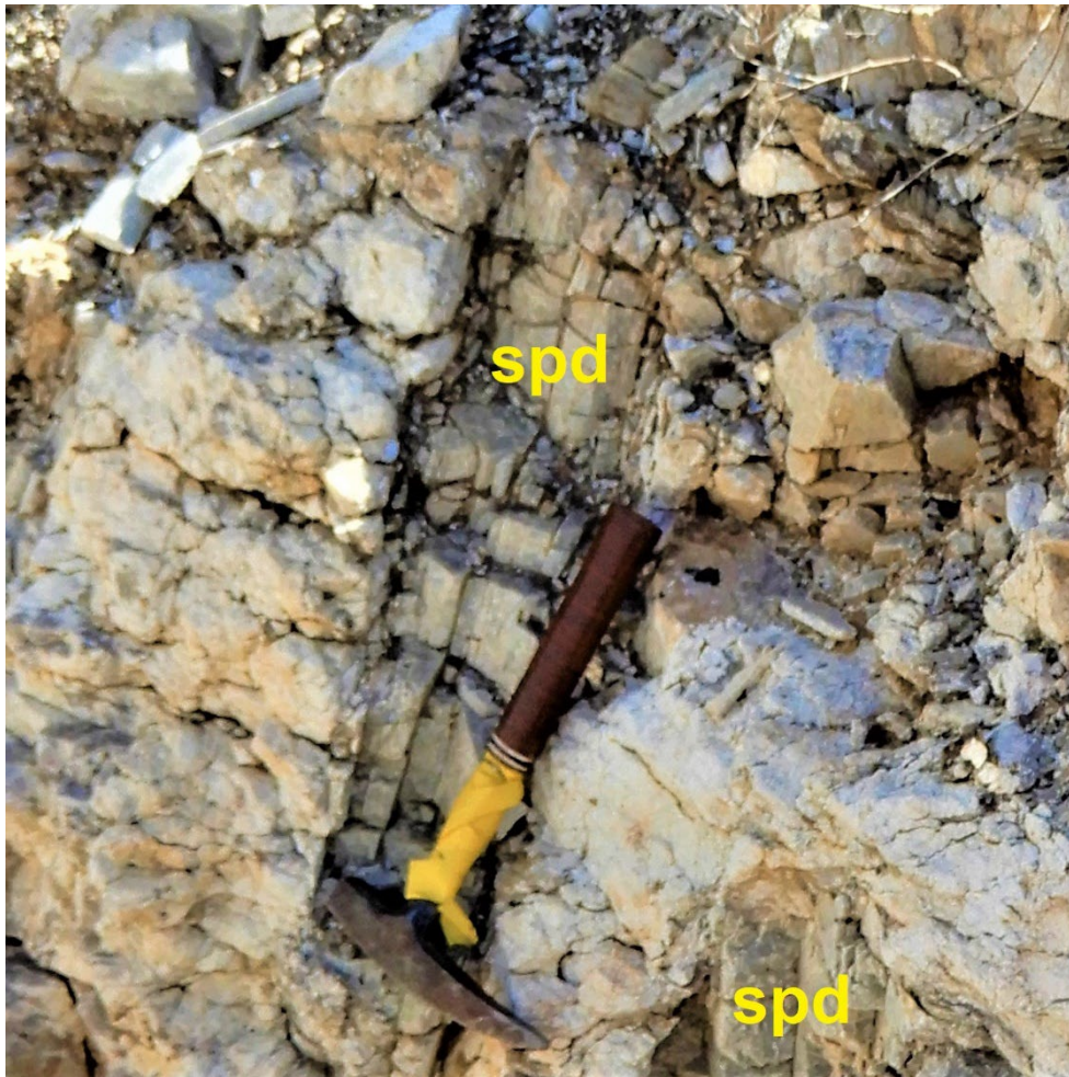
Figure 5: Spodumene crystals, labelled spd , exposed at 226120mE/8323015mN (WGS-84 z33L) in wall of a small trench in a pegmatite within the Namibe Lithium Project.
