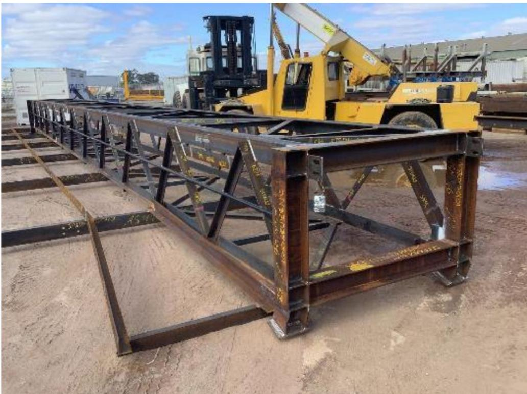
**Figure 9** – Conveyor truss fabrication in Perth.
