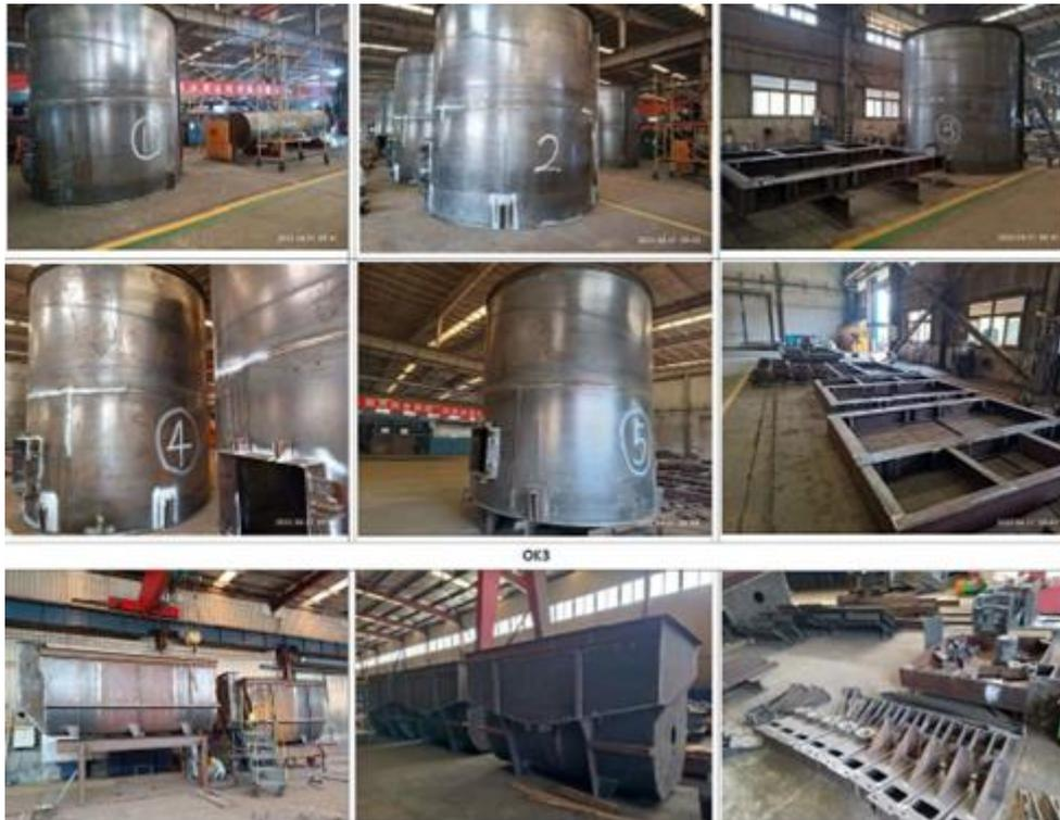
**Figure 10** – Flotation cell fabrication.
