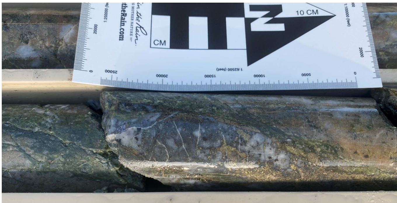
Figure 2 22NGD106 (depth: 69.1m): Highly mineralised steep dipping quartz vein with semi massive pyrite, galena, arsenopyrite, sphalerite and chalcopyrite (centre to right image) and with mineralised breccia fill comprising fine blackish sulphides and chlorite (left part of image); in altered quartz feldspar granite porphyry.
