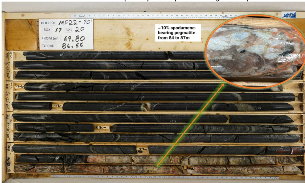
Figure 5: White to grey pegmatite hosts approximately 10% of medium to large, white grey, spodumene crystals intersected from 84-87 metres downhole in Hole MF22-70 (Hole 11). Close ups illustrate significant spodumene mineralisation
