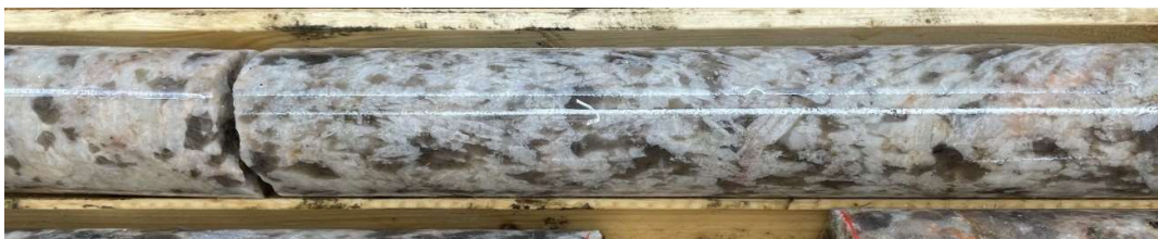
Figure 1: Close up images of large white-cream coloured spodumene crystals intercepted in Hole MF22-72 (Hole 13)
