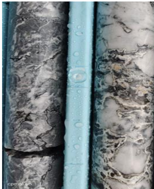
Figure 6: Portion of core in BKDDH-16 showing intense hydrothermally altered limestones.
