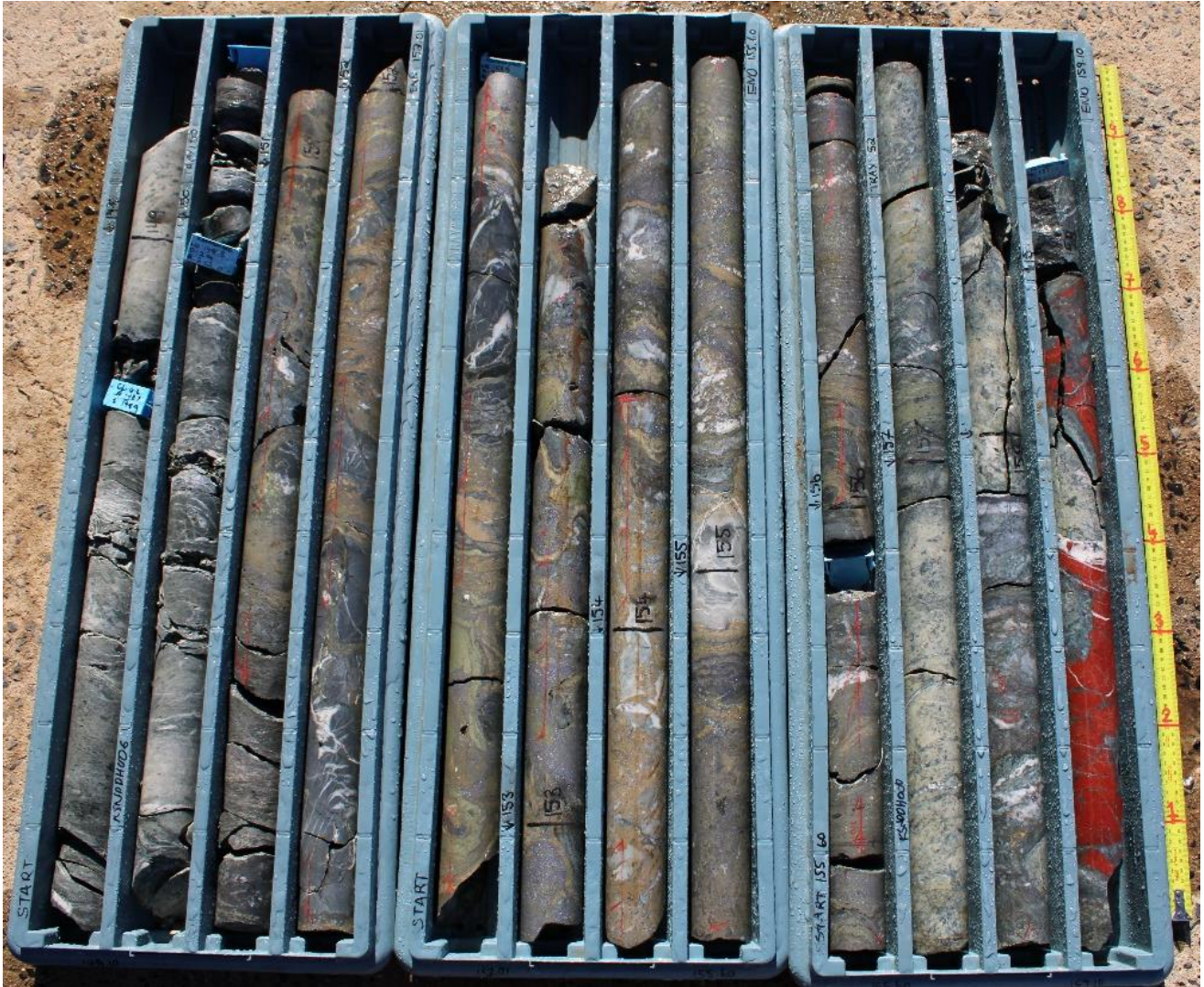
Figure 5: Core Photo of massive sulphide intercept in KSNDDH0006 (150.5m to 156.5m)
