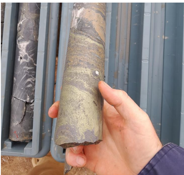
Figure 6: Close up of massive sulphides in HQ3 core in KSNDDH0006 at 152.20m
