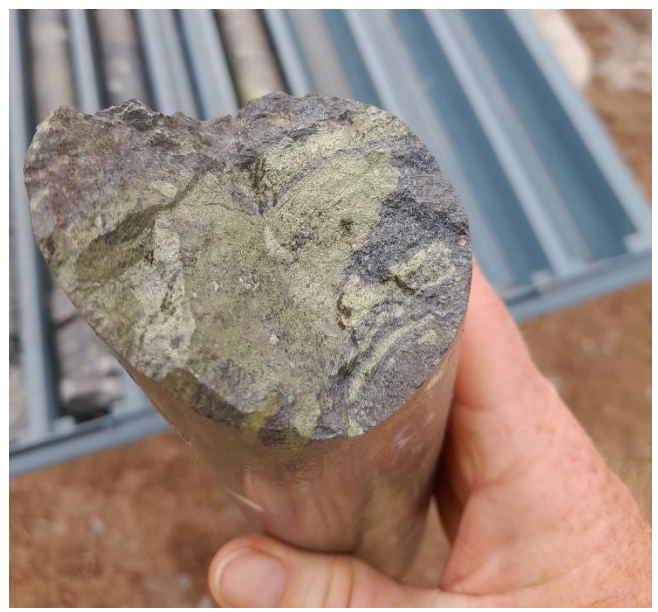
Figure 5: Core Photo of massive sulphide intercept in KSNDDH0006 (150.5m to 156.5m)
