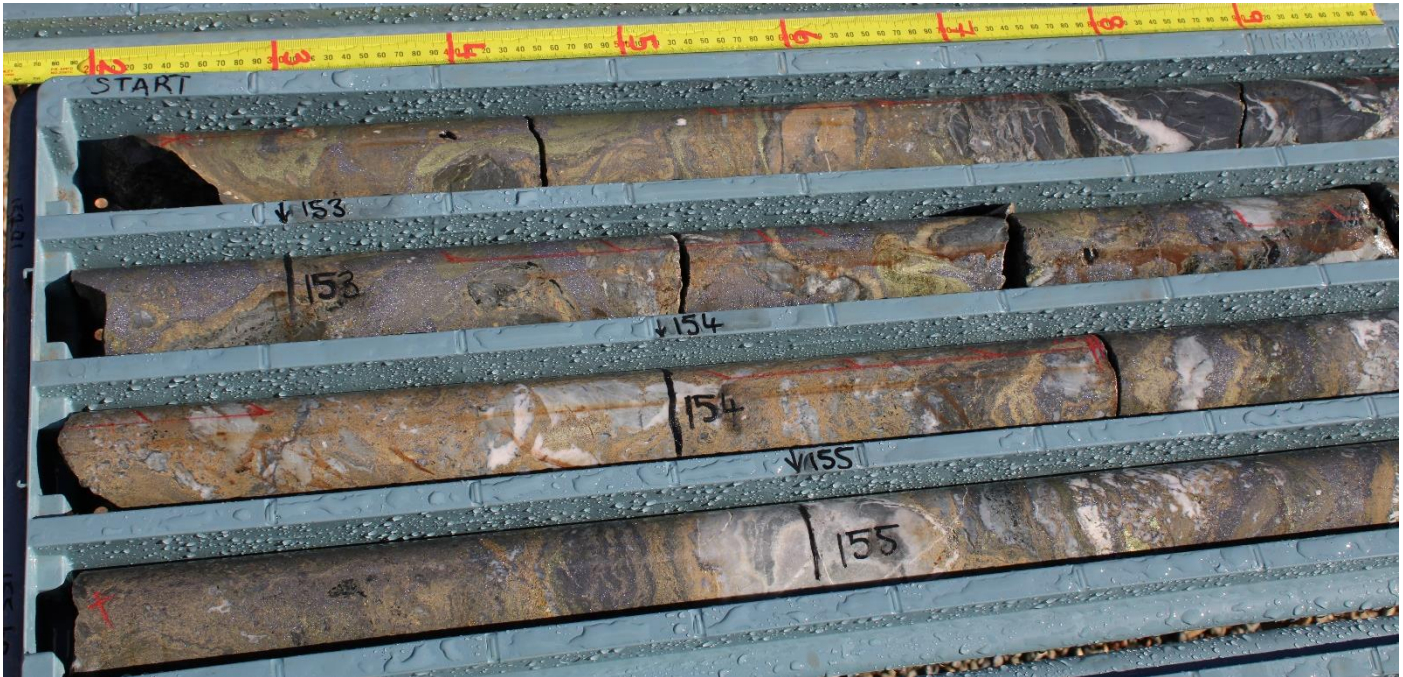
Figure 7: Close up Core Photo of massive sulphide intercept in KSNDDH0006
