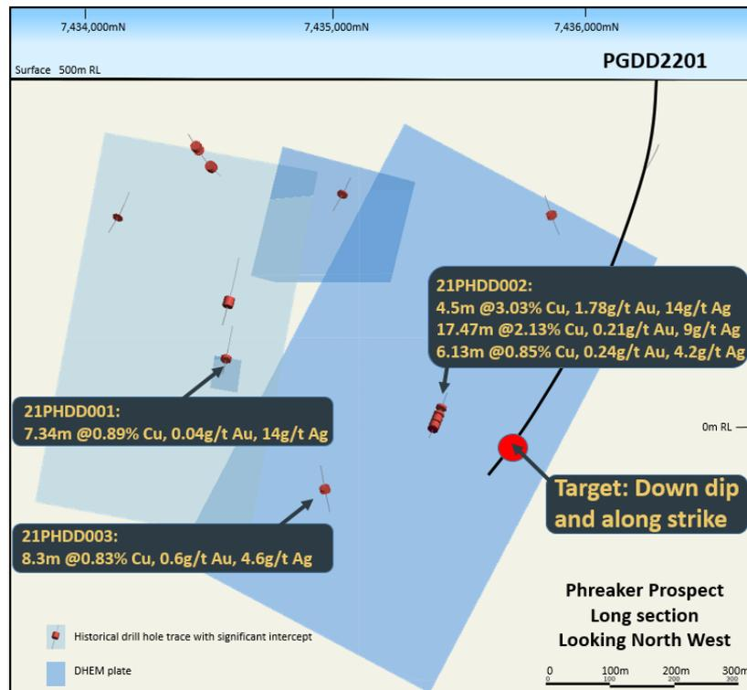
Figure 3 – PGDD2201 (currently drilling) with reference to significant intercepts from 2021 diamond drilling at Phreaker<sup>2</sup>
