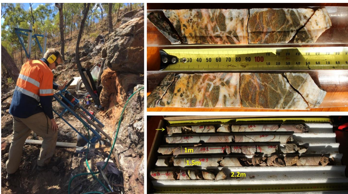
Figure 10. Diamond drilling of the Tornado quartz breccia vein by Placer Gold.
