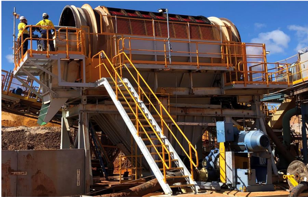
Image 1: The operating feed trommel
