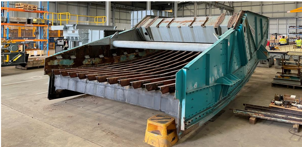
Image 3: The Schenck screen being refurbished at RCR
