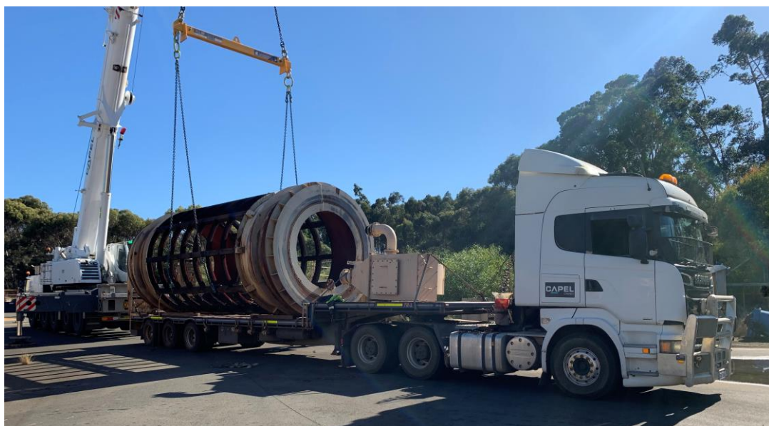
Image 2: The trommel barrel is loaded for transport
