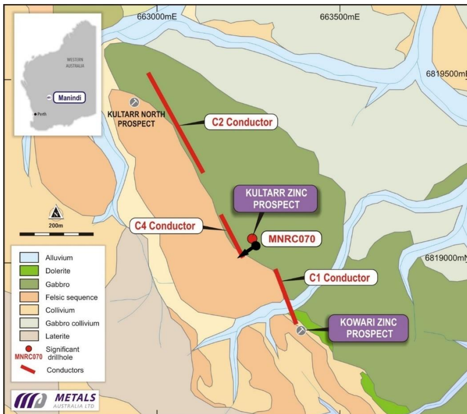
Figure 3: Manindi Zinc Project. Kultarr and Kowari Prospects with projected EM conductors and latest drilling
