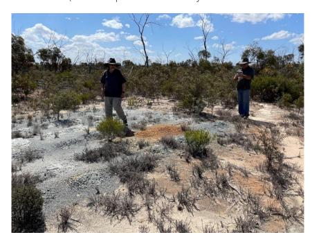
Photo of drill spoil from hole LTRC001 showing high sulphide zones (weathered to orange) correlating with elevated gold to 0.2g/t Au.
