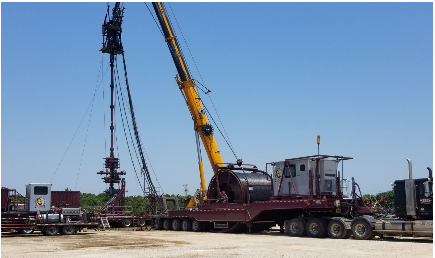
Figure 2. Coiled tubing unit pressure testing the well Christmas tree
