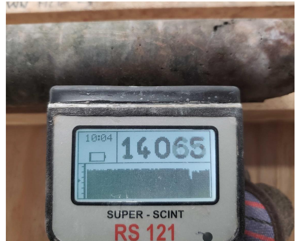
Image: GEM22-019 – RS-121 Hand-held Scintillometer and uranium mineralisation
