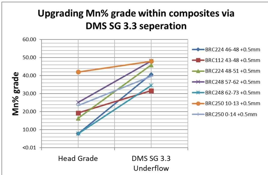
Figure 2: Chart showing upgrade of manganese composite samples by DMS from historical Test
