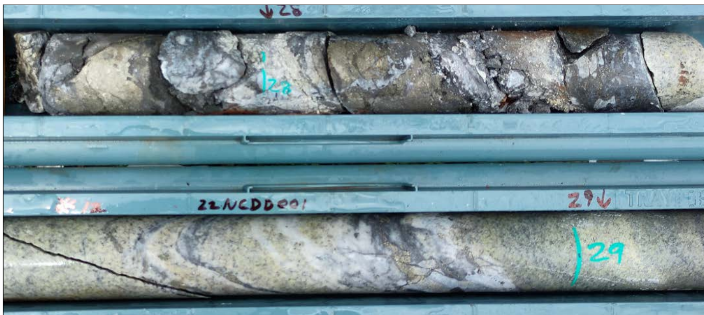
Figure 2. Sulphide-rich mineralised position in diamond hole 22NCDD001 (28m - 29m).
