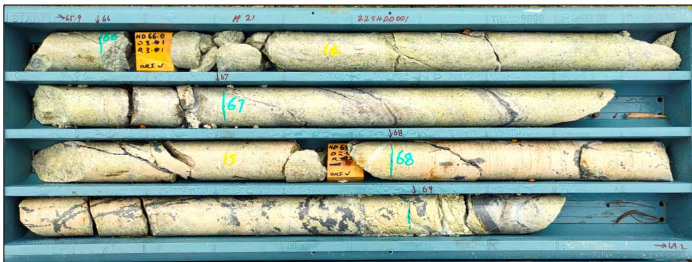
Figure 1. Broad altered and mineralised interval from diamond drill hole 22SHDD001 (65.9m – 69.2m).
