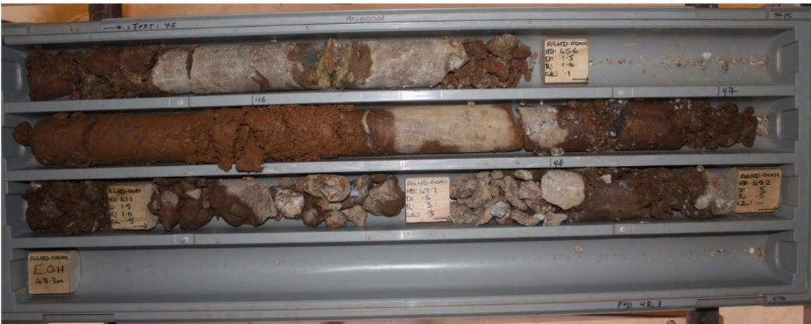
*Figure 3b: The drilled equivalent of the above “cave-fill”, AGHD0001 45.0-48.3m, characteristic “plates” of silica “floating” in a fine matrix of dark red haematitic “mud.”*
