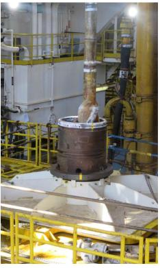
Installation of the bottom hole drilling assembly within the well head housing on the mudmat.
