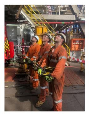
Crew on rig floor of the Valaris MS-1 constructing the bottom hole assembly for drilling of Sasanof-1
