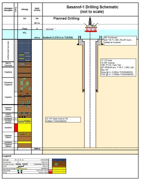
Sasanof-1 Drilling Schematic
